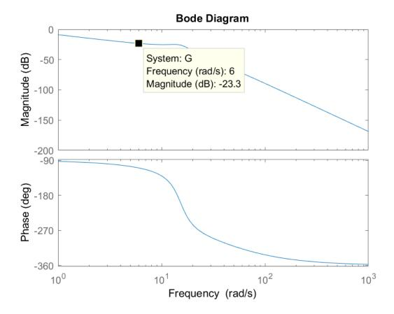
Using the *Data Cursor* tool, we can see that at 6 rad/s, the amplitude is 23.3 dB under the zero axis. As a result, we need to design  $k_p$  such that it lifts the plot 23.3 dB upper.
