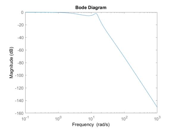
The bandwidth is defined for the value at which the system reaches the magnitude of -3dB. As a result, we can confirm the previous value by zooming on the graph.
