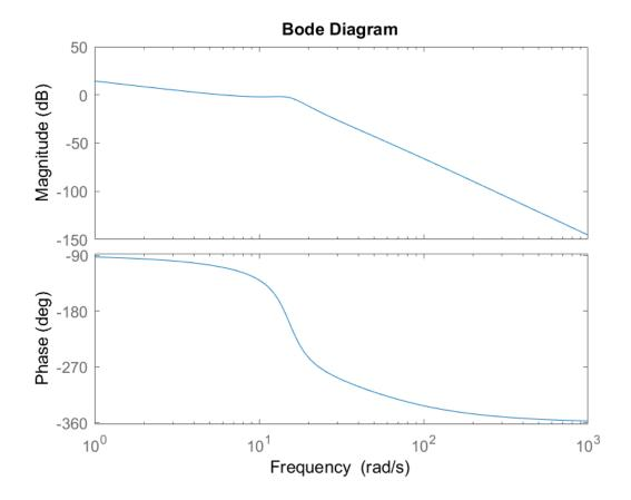
The phase margin on the plot can be red by measuring the distance between the graph at the crossover frequency  $(6 \ rad/s)$ and  $-180^{\circ}$ . Using the same strategy, we can read the gain margin counting the difference between the actual position of the plot and 0dB at the frequency where the phase crosses the  $-180^{\circ}$  horizontal line (around  $14.5 \ rad/s$ ):
