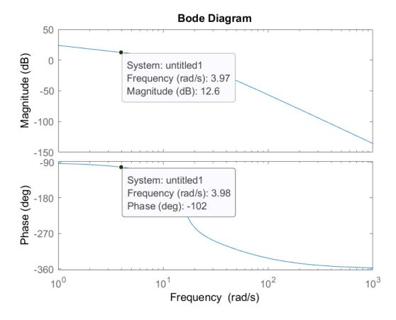
As presented on the previous diagram, the graph need to be shifted around  $-12.6 \ dB$  upward to respect the desired qualifications. We can see that the phase margin is around  $78^{\circ}$ , which is already greater than  $55^{\circ}$ . As
