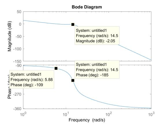
We can compare the Gain and Phase margins appearing on the plot by computing the matlab command:
