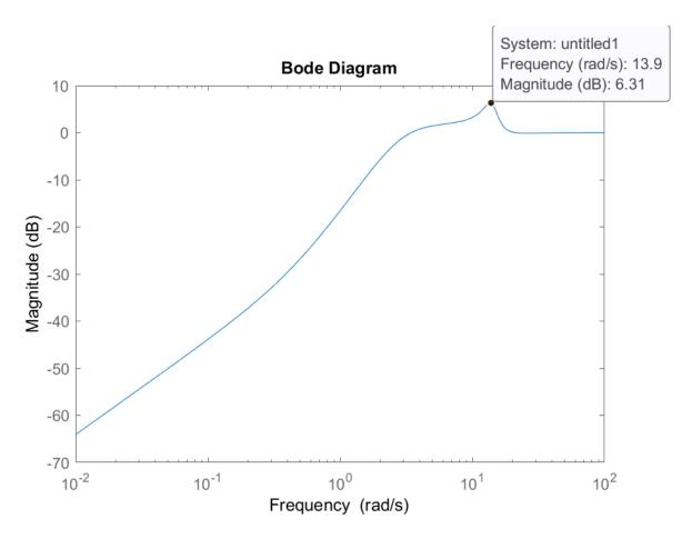
The *Modulus Margin* is computed by taking the inverse of the peak value red on the previous plot (note that the value should be converted from decibel to standard units):  $MM = \frac{1}{10^{\frac{6.31}{20}}} = 0.484$
