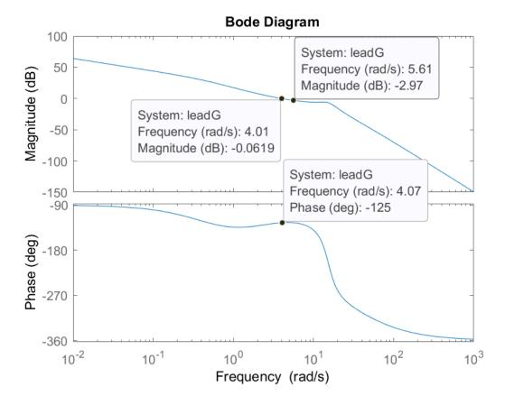
The closed-loop bandwidth is defined as the frequency where the graph reaches the -3 dB value. We can read the bandwidth directly on the graph:  $BW = 5.61 \ rad$ .
